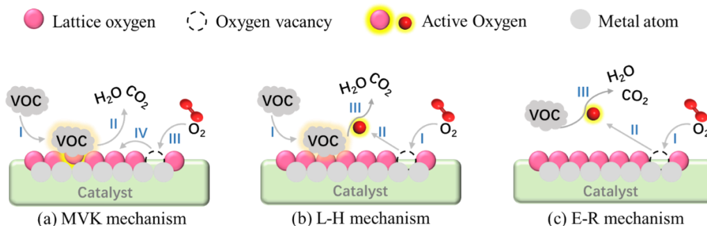
Fig. 1.2. Schematic diagrams of degradation mechanisms for VOCs oxidation: (a) MVK, (b) L-H and (c) E-R mechanisms.
