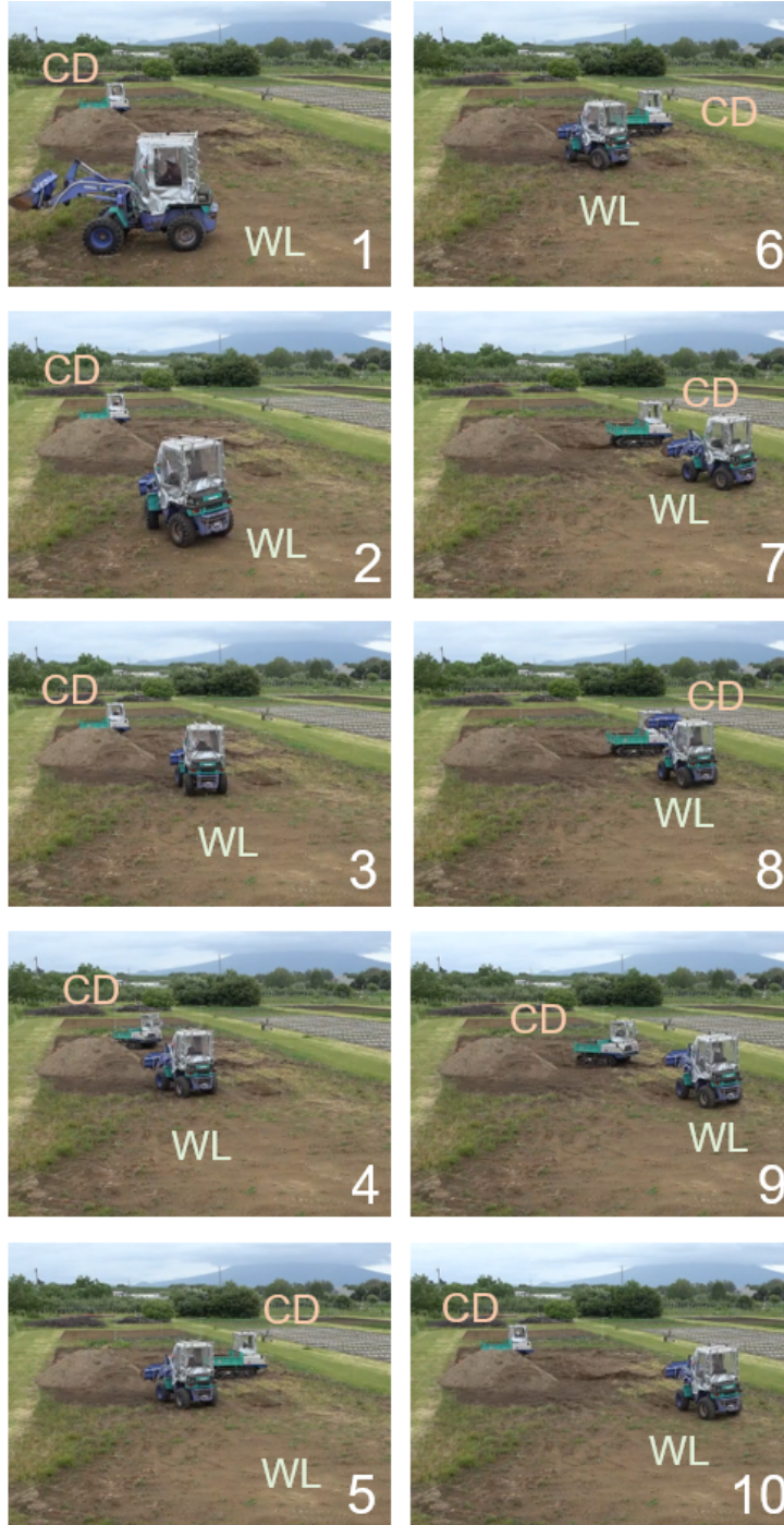
Fig. 3.29: Construction machines that perform a series of tasks (Adapted from [3]).
