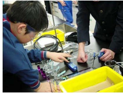
Fig. 10 – Measurement of absorbance of solution treated with a chemical reagent
