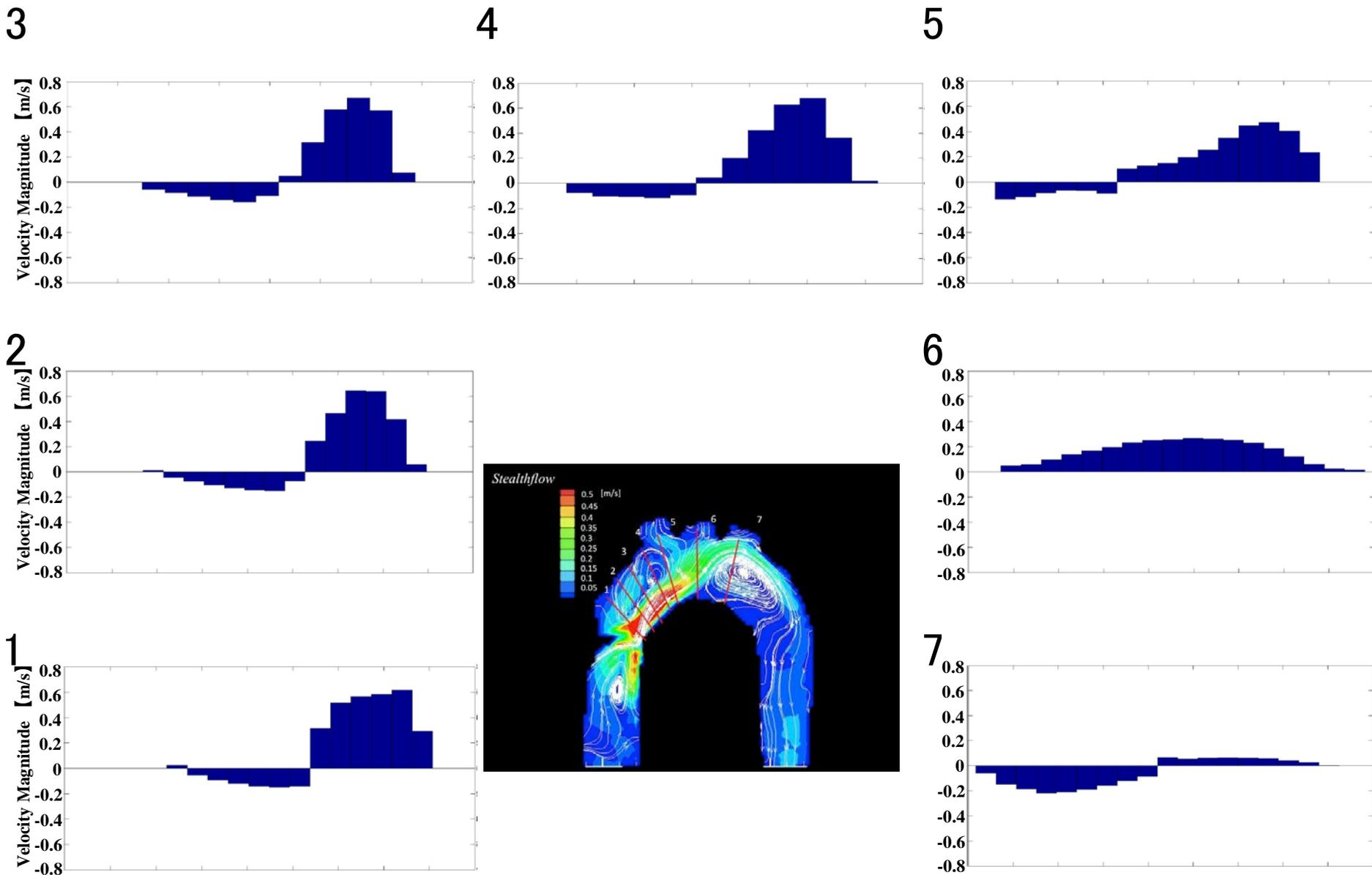
Fig. 6. Histogram of longitudinal flow components along the center of the aorta in each axial section in Stealthflow cannula.
