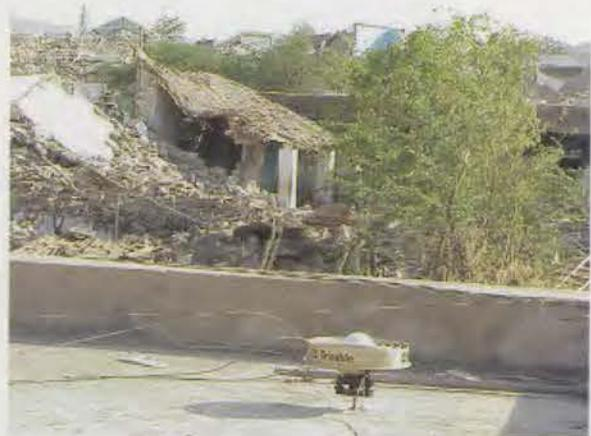
Photo 4.1 GPS antenna installed on a roof-top of a building in Lodai (S8), which was not collapsed by the earthquake. The background shows completely destroyed houses (page 46).
