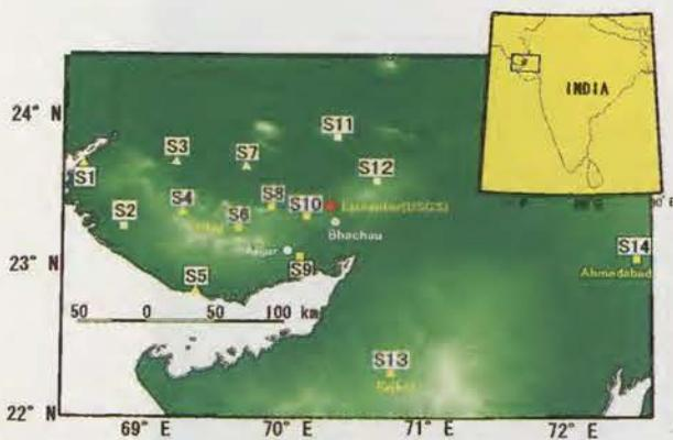
Figure 4.1. GPS network consisting of 14 re-observable stations (S1-S14). Red star denotes the epicenter determined by USGS (page 46).
