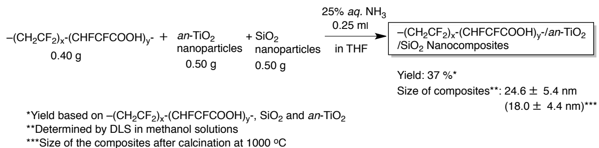
Scheme 1-3 Preparation of \text{-(CH}_2\text{CF}_2\text{)}_x\text{-(CHFClFCOOH)}_y\text{-an-TiO}_2\text{/SiO}_2 nanocomposites.
