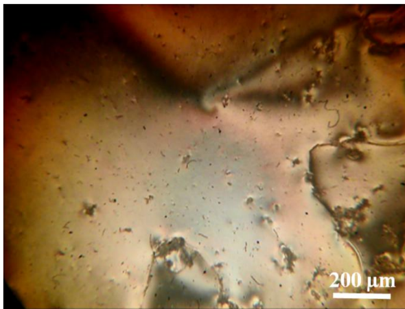
Fig.3– 18 (a) Polarized optical texture of V-(7,7) on a glass plate without a cover glass in the N phase. (b) Polarized optical texture in the N phase just above the DC phase. The circle indicates the appearance of the transient state.
