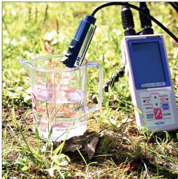
Figure 3–3. Measurement method of stream water pH. (a): Photograph measuring pH directly. (b): Photograph measuring pH using beaker.
