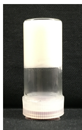
Figure 4-8 Gelation of water by using the R_F-(VM-SiO_2)_n-R_F/Glu-SiO_2 nanocomposites (Run 9 in Table 4-3).
