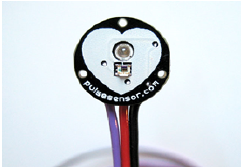
Fig. 6.3: Pulse sensor (SEN-11574, SparkFun Electronics) used to obtain PPG signal.
