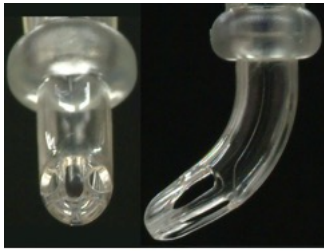
Fig 32. Edwards EZ glide cannula. The cannula tip is curved (45 degrees). Cannula exit creates a pentagonal outlet with the mainstream on the lesser curvature of the cannula tip. It creates flame-shape flow from the exit.
