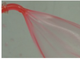
Fig 32. Edwards EZ glide cannula. The cannula tip is curved (45 degrees). Cannula exit creates a pentagonal outlet with the mainstream on the lesser curvature of the cannula tip. It creates flame-shape flow from the exit.
