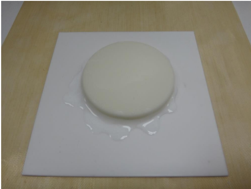
Fig. 18 Cap sealed by Al 2 O 3 -water solution
